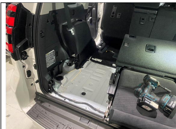
STEP 1.13 THE PASSENGER SIDE 3 RD ROW SEAT CAN NOW BE COMPLETELY REMOVED. PULL OUT AND SET ASIDE.
