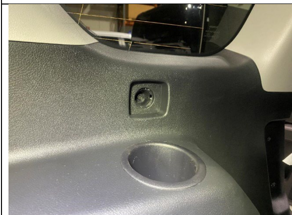
STEP 1.17 REMOVE PLASTIC COVER AS SHOWN AND REMOVE M6 SCREW AS SHOWN.
