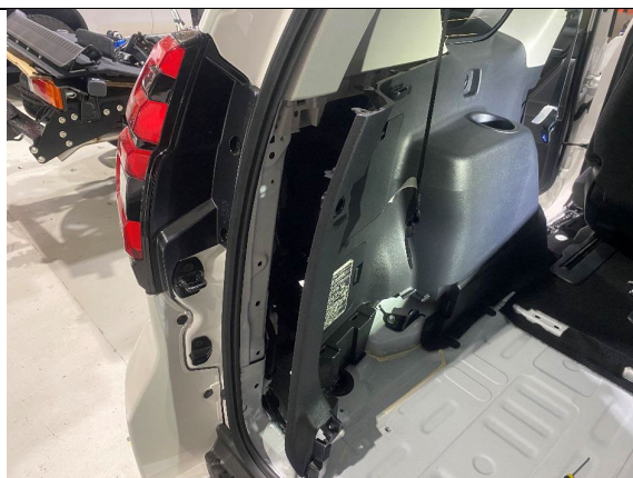
STEP 1.18 PULL BACK RUBBER SEAL AND BEGIN PULLING BACK QUARTER PANEL AS SHOWN. CHECK FOR TRIM CLIPS AGAIN.
