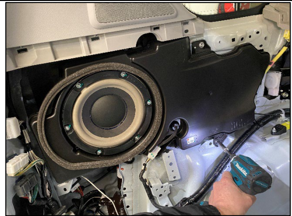
STEP 2.2 REMOVE THE 4 X M6 SCREWS AND KEEP SPEAKER ASIDE. SCREWS NOT REQUIRED LATER INSTALL, KEEP WITH SPEAKER.
