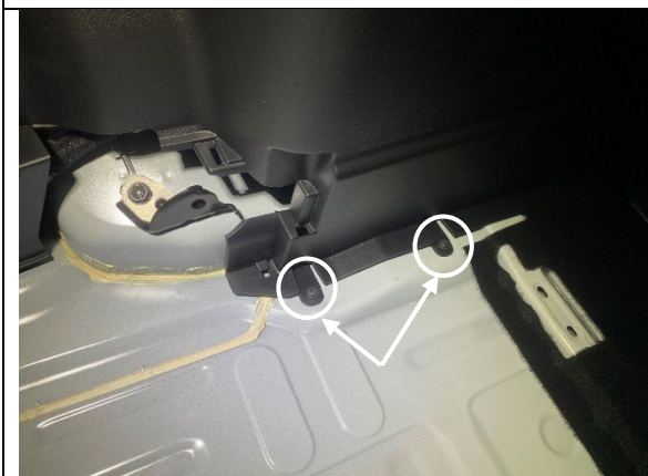
STEP 1.15 REMOVE 2 X PHILLIPS HEAD SCREWS AT BASE OF REAR QUARTER PANEL.
