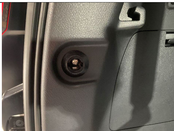
STEP 1.16 TWIST REAR PLASTIC CAP 90 DEGREES AND REMOVE. REMOVE M6 PHILLIPS HEAD SCREW EXPOSED.
