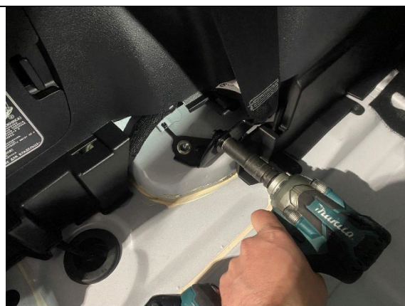
STEP 1.14 REMOVE 14MM BOLT ON SEAT BELT AS SHOWN.
