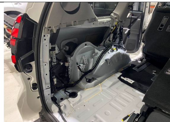
STEP 1.20 FULLY REMOVE QUARTER PANEL GENTLY AND SET ASIDE. CHECK FOR TRIM CLIPS (REFER TO STEPS 1.21-1.23 BELOW)
