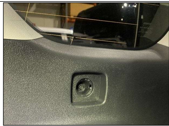
STEP 1.2.12 REMOVE PLASTIC COVER BELOW WINDOW AS SHOWN AND REMOVE M6 SCREW IN CAVITY.
