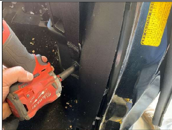
STEP 1.2.7 REMOVE THE SECOND ROW SEAT BELT USING 14MM SOCKET AS SHOWN.
