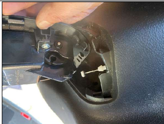
STEP 1.2.9 FLIP THE ASSEMBLY OVER AND RELEASE THE CABLE AS SHOWN. TAKE NOTE OF THE ORIENTATION FOR RE-INSTALLATION LATER.
