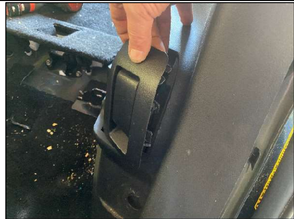
STEP 1.2.8 POP THE SEAT FOLD LEVER ASSEMBLY OUT AS SHOWN.
