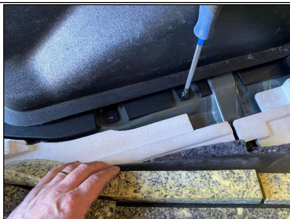
STEP 1.2.11 PULL THE CARPET BACK AND REMOVE 2 X PHILLIPS HEAD SCREWS.
