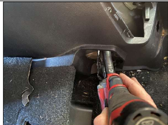
STEP 1.2.10 REMOVE BOTTOM BOLT AS SHOWN.
