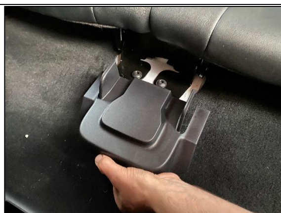
STEP 1.18 REMOVE THE CENTRE COVER BY PULLING TOWARDS THE FRONT OF THE VEHICLE. (CHECK FOR CLIPS) AND REMOVE PASSENGER SIDE T50 BOLT.
