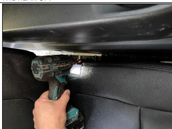
STEP 1.17 REMOVE THE T50 BOLT FROM BETWEEN THE SEAT, YOU MAY NEED A SHORT EXTENSION TO ACCESS THIS BOLT.
