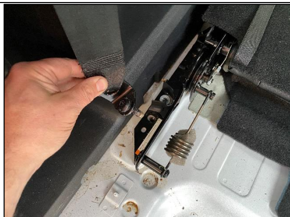
STEP 1.13 REMOVE THE PASSENGER SIDE SEAT BELT BOLT USING T50 TORX BIT.
