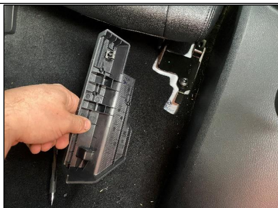
STEP 1.15 MOVE BACK TO THE 2 ND ROW SEAT DOOR AND FOLD THE 3 RD ROW SEAT BACK UP. REMOVE PLASTIC TRIM COVER, PULL TOWARDS FRONT OF CAR TO SLIDE OVER TAB THEN LIFT THE REAR UP.
