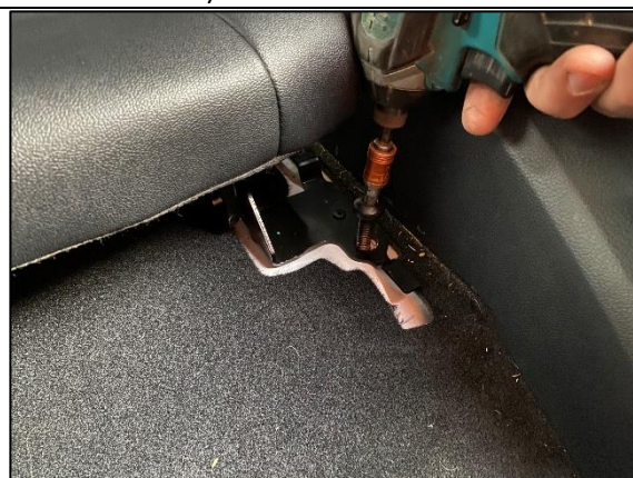
STEP 1.16 UNDO T50 BOLT EXPOSED FROM STEP 1.15.
