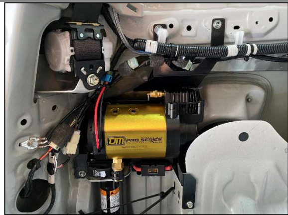
STEP 3.2 BOLT INTO 4 X CAPTIVE NUT LOCATIONS USING M6 X 20 SEMS ASSEMBLY BOLTS .
