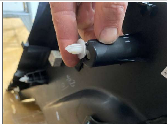
STEP 1.12 REFERENCE PIC FOR TRIM CLIPS- CHECK ALL REMOVED PANELS FOR TRIM CLIPS AND RE-INSERT IF THEY HAVE PULLED OUT.
