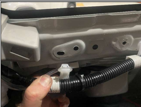
STEP 1.11 REMOVE THE PLASTIC CLIP ON THE BODY LOOM BELOW THE WINDOW AS SHOWN.
