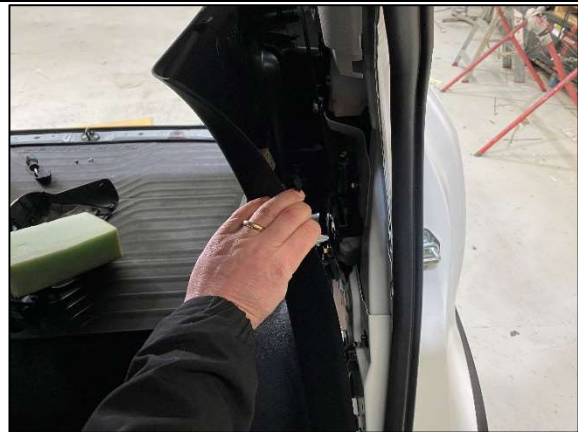
STEP 1.8 MOVE BACK TO THE SECOND ROW OF SEATS PASSENGER SIDE DOOR, PULL BACK RUBBER AND START PULLING BACK QUARTER PANEL CLIPS.
