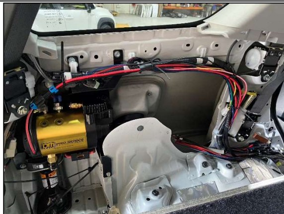
STEP 3.3 CABLE TIE NEATLY ALL WIRING AND HOSES.
