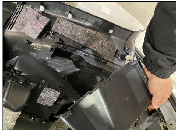
STEP 1.10 UNSCREW REAR STORAGE COMPARTMENT SCREWS AS SHOWN AND REMOVE.
