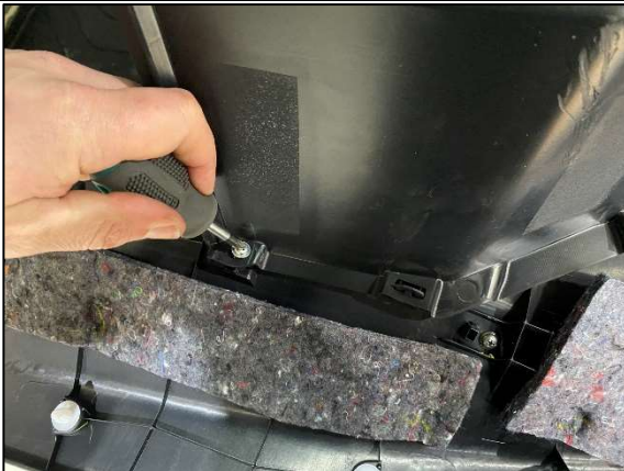
STEP 1.9 REMOVE THE QUARTER PANEL FROM THE VEHICLE AND SIT ON A SOFT CLEAN SURFACE.
