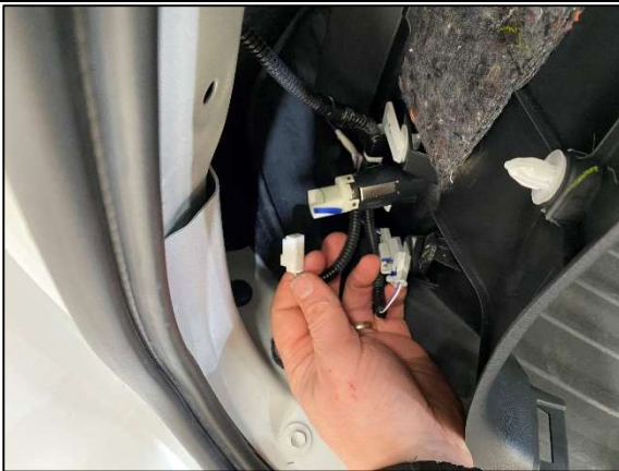
STEP 1.7 UNPLUG POWER SOCKET AS SHOWN.
