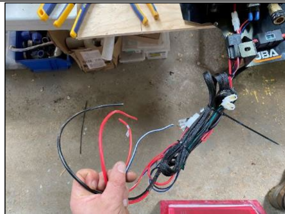
STEP 2.9 NEATLY FOLD THE LOOM AND CABLE TIE AS SHOWN LEAVING ABOUT 30-40CM OF THE MAIN POWER/NEG WIRE AND THE RED/YELLOW ACC POWER/BLUE WHITE DASH WIRES OUT AS SHOWN.
