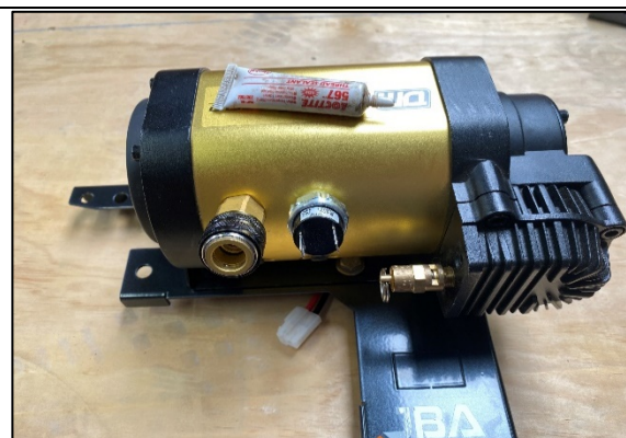
OPTIONAL STEP 2A.2-2 FIX THE NITTO FITTING TO THE COMPRESSOR TOP 1/4" BSP LEFT SIDE THREAD AS SHOWN.
