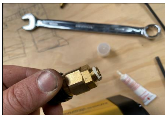
OPTIONAL STEP 2A.2-1 APPLY 567 THREAD SEALANT TO THE NITTO FITTING.
