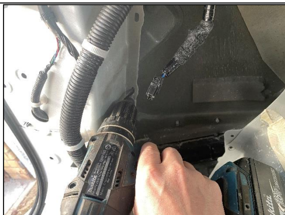
STEP 1.21 PULL BACK THE 3 X PLASTIC RETAINING CLIPS HOLDING IN THE MAIN BODY LOOM DRILL OUT THE MIDDLE SLOTTED HOLE ON THE LEFT HAND SIDE TO 12MM AS SHOWN
