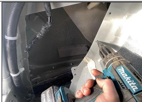
STEP 1.20 DRILL OUT THE MIDDLE HOLE IN THE POSITION SHOWN TO 12MM.
