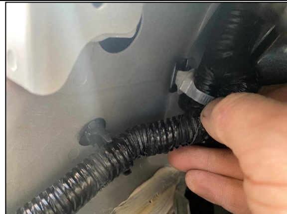
STEP 5.8 RE-CLIP THE BOTTOM CLIP TO THE TAB ON THE JBA COMPRESSOR BRACKET AS SHOWN
