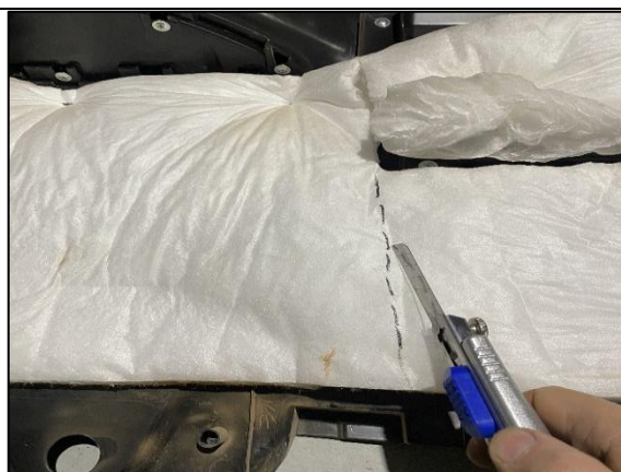
STEP 1.24 MARK AND TRIM THE SOUND DEADENING ON THE REAR QUARTER PANEL AS SHOWN.
