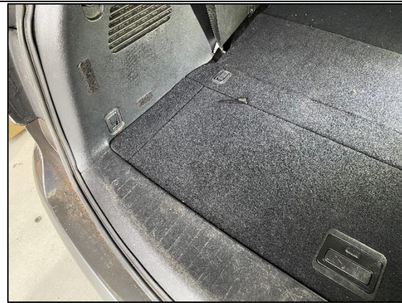
STEP 5.10 REFIT REAR QUARTER PANEL AND SEATS REFERING TO STEPS 1.1-1.22 ABOVE IF REQUIRED. VACUUM AND WIPE DOWN ALL SURFACES.
