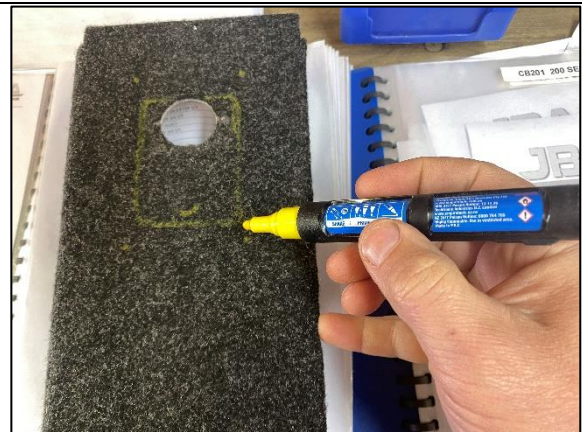
STEP 2 MARK OUT A SQUARE AROUND THE SWITCH AND AIR OUTLET AND ADD 3-4MM FOR CUTTING GUIDE.
