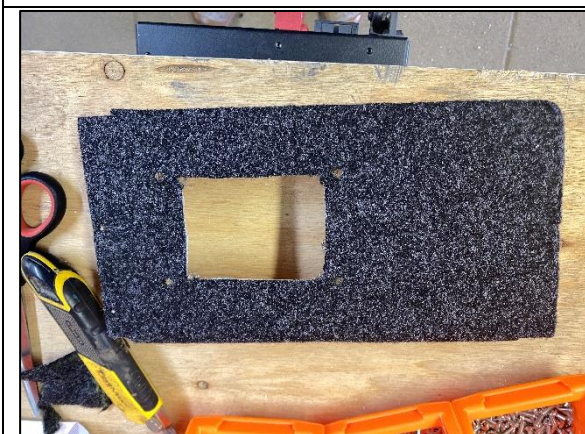
STEP 5 CLEAN UP ANY SWARF AND DEBUR THE EDGES OF THE HOLE CUT.
