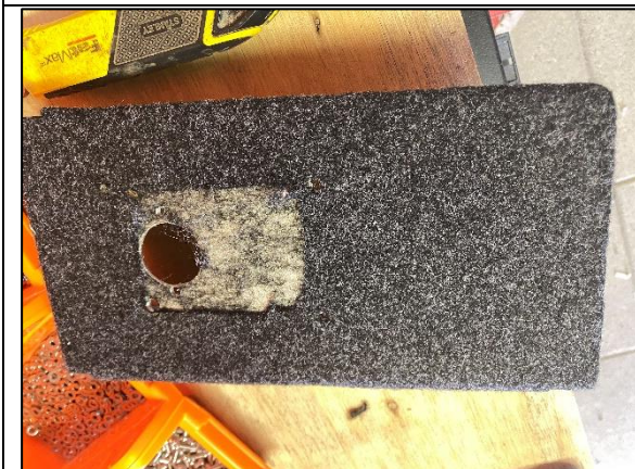
STEP 3 DRILL OUT THE 4 OUTER HOLES (CAN BE DRILLED TO 5-6MM FOR ANY ADJUSTMENTS AND DRILL A HOLE IN EACH CORNER OR THE MARKED CUTTING GUIDE. CUT OUT THE CARPET TO MAKE THE NEXT STEP EASIER.
