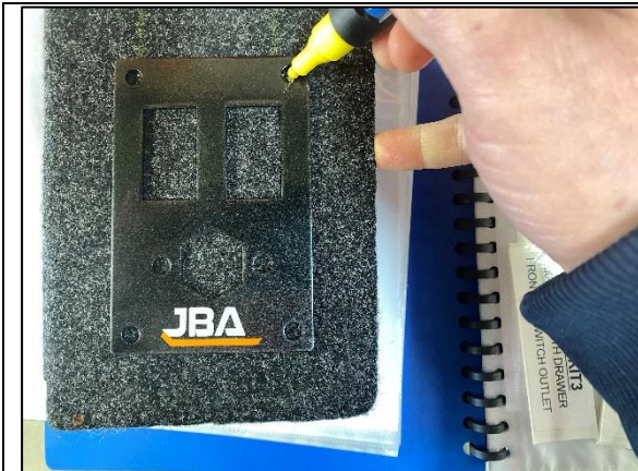
STEP 1 PLACE THE MOUNTING PLATE IN THE DESIRED LOCATION AND MARK THE 4 HOLES AND OUTLET LOCATIONS AS SHOWN.
