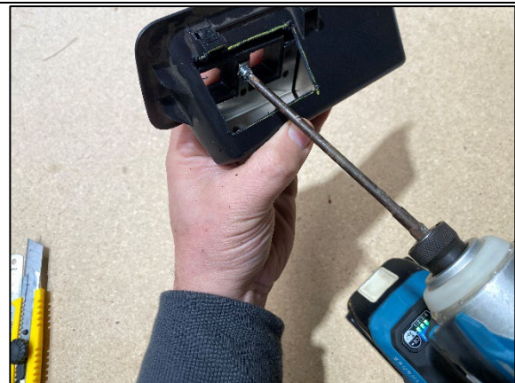
STEP 3.3.8 USE 1-2 M4 X 10 DOME HEAD SCREWS FINGER TIGHT TO TEMPORARILY MOUNT THE SWITCH BLOCK IN PLACE.
