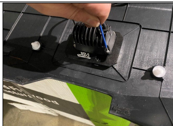
STEP 2.6 RE INSTALL 4 X 2.5MM SCREWS REMOVED IN STEP 2.1 AND ENSURE LIGHT IS SITTING FLAT AND TIGHT.
