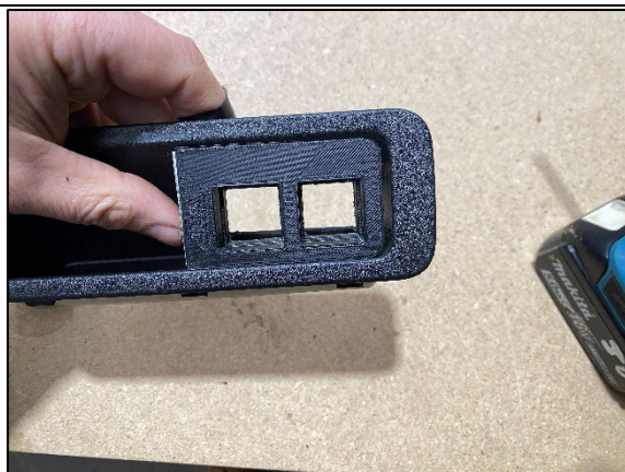
STEP 3.3.9 ADJUST THE SWITCH BLOCK AND PLATE TO LINE UP GAPS EVENLY.
