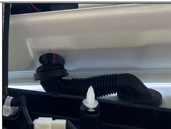
STEP 5.1 PULL DOWN THE TOP SECTION OF THE RUBBER BOOT AS SHOWN.
