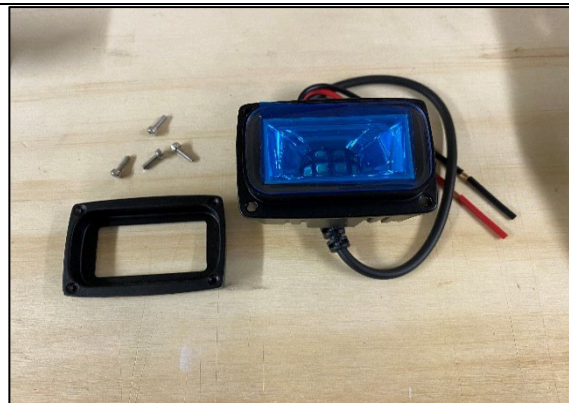
STEP 2.2 SEPARATE THE FRONT METAL FASCIA AND DISCARD (KEEP THE SCREWS AND PLASTIC LENS).
