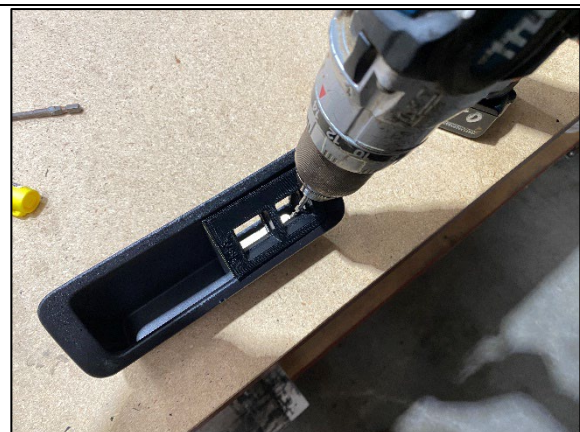
STEP 3.3.10 CAREFULLY PILOT DRILL THE 4 HOLES IN THE SWITCH BLOCK PLATE AS SHOWN.
