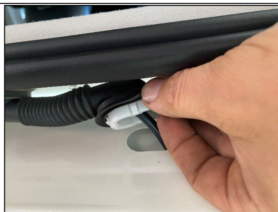
STEP 5.2 IT IS EASIER TO ALSO REMOVE THE BOTTOM SECTION TO FEED THE WIRE THROUGH BUT THE BOTTOM SECTION CAN BE MORE DIFFICULT TO RE-INSTALL TO THE VEHICLE. THE BOTTOM SECTION HAS A WHITE PLASTIC RETAINER THAT IS EASIER IF YOU REMOVE THIS BY PUSHING THE SIDE TABS IN. IF THE BOOT COMES OFF THE WHITE CLIP, IT CAN BE DIFFICULT TO RE-INSTALL THE BOOT BACK ON.
