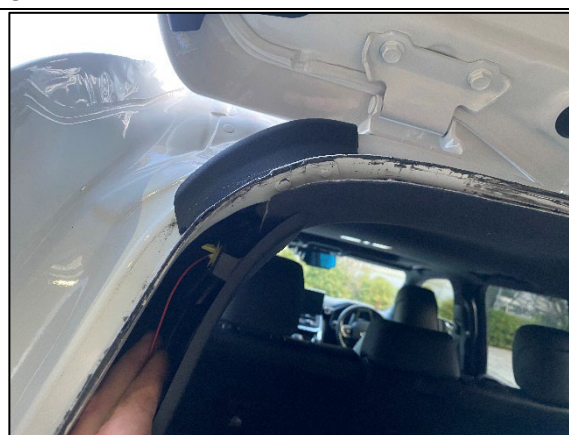
STEP 5.4 REMOVE THE RUBBER SEAL AROUND THE BOOT AREA AND PULL THE PANELS AND TRIMS BACK JUST ENOUGH TO RUN THE WIRING HARNESS THROUGH. ENSURE NOTHING IS PINCHED OR CAUGHT.
