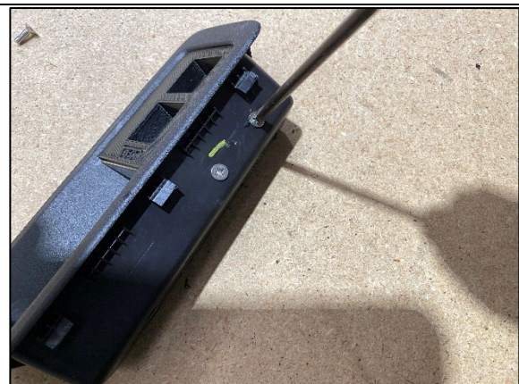
STEP 3.3.12 USE THE 4 X M4 X 12 CSK HEAD SCREWS AND FLANGE NUTS TO FULLY INSTALL THE SWITCH PLATE. USE THE 4 X M4 X 10 DOME SEMS TO ATTACH THE BLOCK TO THE PLATE IN THE CAPTIVE POINTS. ADJUST ALL GAPS AS NEEDED AND FULLY TIGHTEN ALL SCREWS ONCE HAPPY.
