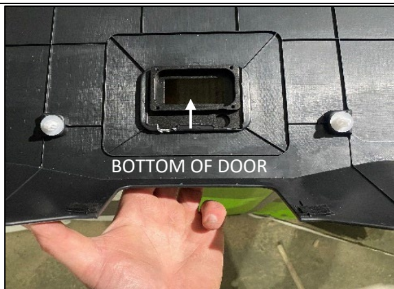
STEP 2.3 PRESS THE JBA FASCIA (JBA-LB804A) INTO THE REAR TAILGATE SECTION AS SHOWN. NOTE THE ORIENTATION, ENSURE THE CUT OUT FOR THE LIGHT IS FACING TOWARDS THE TOP AS SHOWN.
