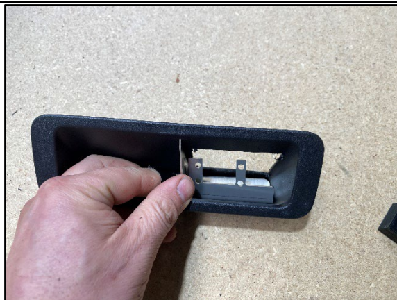
STEP 3.3.7 PLACE JBA-LB804SH SWITCH BLOCK PLATE INTO THE HANDLE.
