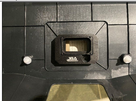
STEP 2.4 PLACE REAR SPACER X 2 (JBA-LB804B) OVER FASCIA AS SHOWN.
