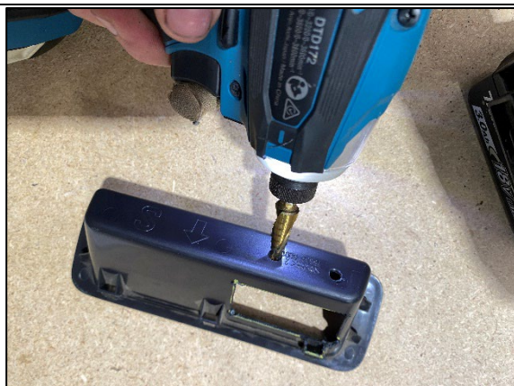
STEP 3.3.11 REMOVE THE SWITCH PLATE AND BLOCK AND DRILL ALL PILOT HOLES OUT TO 5MM.
