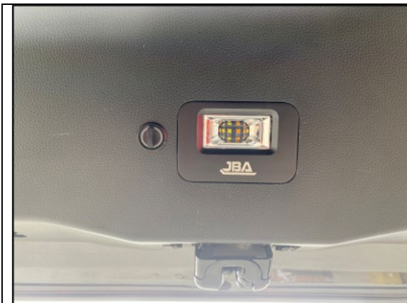
STEP 3.1.1 THE FINAL LOCATION OF THE SWITCH SHOWN FOR REFERENCE.
