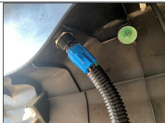
STEP 3.2.6 CONNECT WIRING HARNESS.
