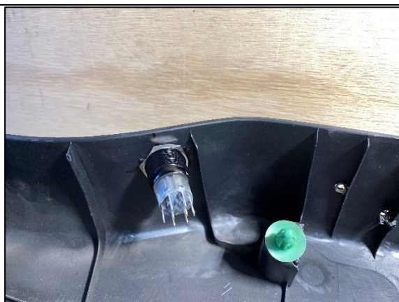
STEP 3.2.5 DRILL THE HOLE OUT 20MM AND INSTALL THE SWITCH WITH NUT FROM REAR AS SHOWN.
