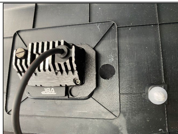
STEP 3.1.3 DRILL THE SWITCH HOLE OUT TO 20MM USING STEP DRILL AS SHOWN. INSERT THE SWITCH AND TIGHTEN NUT FROM BEHIND.
