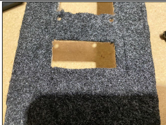
STEP 3.2.3 USE THE APPROPRIATE TOOL (SUGGEST JIGSAW FOR ALUMINUM AND ANGLE GRINDER FOR STEEL) TO CUT THE SECTION OUT AND FILE BACK EDGES AND CARPET.
