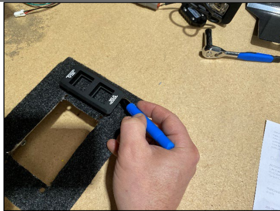
STEP 3.2.1 CHOOSE THE DESIRED LOCATION ON THE DRAWER FRONT AND MARK THE BASE.
