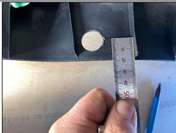
STEP 3.2.3 MARK THE CENTRE 20MM FROM THE BOTTOM LIP.
