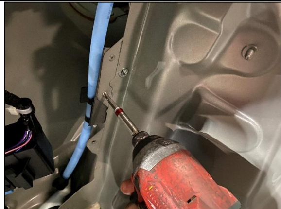
STEP 1.4.8 INSTALL 10-CB222BR-E HOSE RELOCATION BRACKET USING M4 X 12 CSK SCREWS AND NYLOC NUTS.
