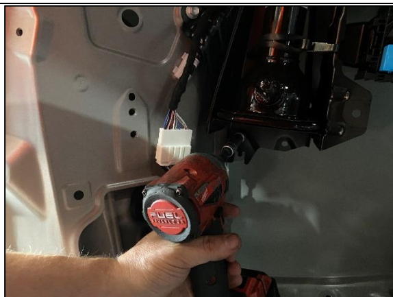
STEP 1.4.1 REMOVE THE BOTTOM LEFT 10MM BOLT FROM THE JACK AS SHOWN.
