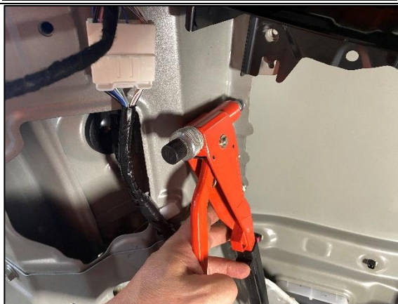
STEP 1.4.6 INSERT M6 CAPTIVE NUTS AS SHOWN INTO PREVIOUSLY DRILLED HOLES.
