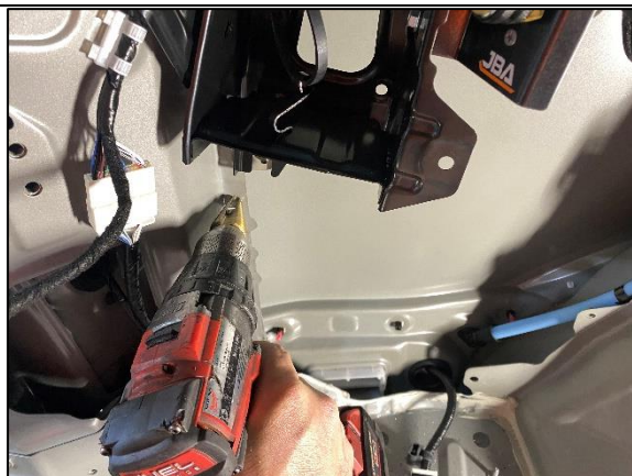
STEP 1.4.5 DRILL OUT THE MARKED HOLES TO 10MM. VACUUM ALL SWARF, DEBUR HOLES AND TREAT WITH ANTI-CORRSION PAINT.
