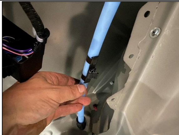
STEP 1.4.7 UNCLIP THE ROOF DRAIN HOSE BRACKET AS SHOWN.
