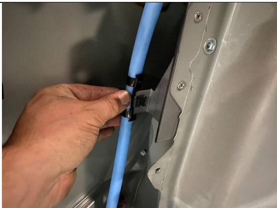
STEP 1.4.9 RE-CLIP THE ROOF DRAIN HOSE TO THE JBA RELOCATION BRACKET AS SHOWN.
