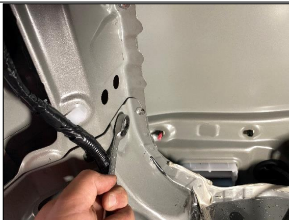
STEP 1.4.4 REMOVE BOTTOM LEFT CAPTIVE BOLT AS SHOWN TO MAKE ACCESS FOR DRILLING HOLE AND NUTSERTING EASIER. DON'T FORGET TO RE-INSTALL AFTER DRILLING.
