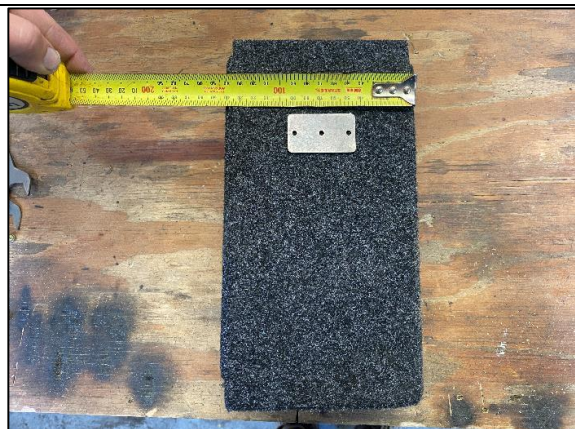
STEP 1 IDENTIFY THE LOCATION FOR THE AIR OUTLET AND MARK WITH TEXTA/SCRIBE. POSITION THE CENTRE HOLE OF THE DRILLING TEMPLATE OVER PREVIOUSLY MARKED POINT.
