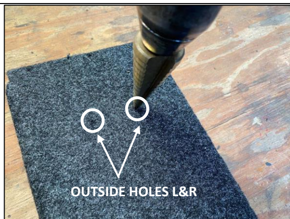
STEP 4 REMOVE THE DRILLING TEMPLATE AND ENLARGE OUTER HOLES (L&R) TO 5MM .
