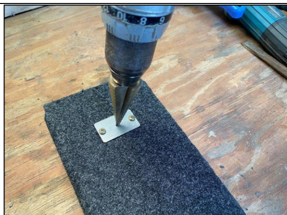
STEP 3 DRILL CENTRE HOLE USING 3-4MM PILOT HOLE.
