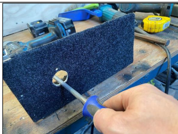
STEP 6 CLEAN ALL HOLES DEBURRING ANY SHARP EDGES USING RAT TAIL FILE.
