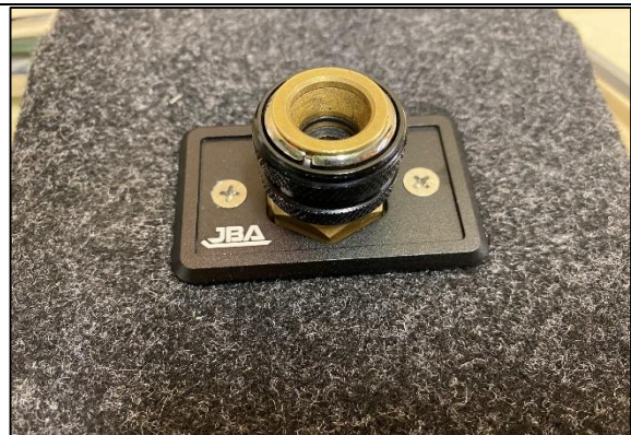
STEP 12 FEED THE BULKHEAD AND NITTO FITTING ASSEMBLY THROUGH THE FACIA AS SHOWN. IF STEP 11 WASN'T COMPLETED PROPERLY, THE BULKHEAD WILL HIT THE HOUSING BRACKET SO CHECK AT THIS POINT AND ADJUST IF NEEDED.
