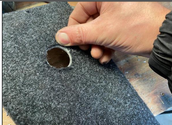
STEP 7 CLEAR OUT ANY SWARF FROM BEHIND CARPET (IF APPLICABLE)
