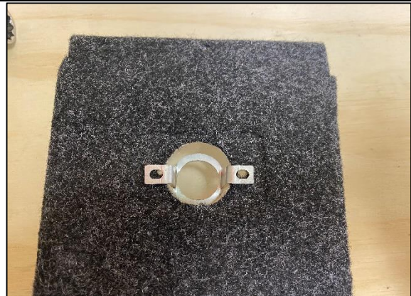
STEP 8 PLACE JBA-CB101B HOUSING BRACKET INTO LARGE CENTRE HOLE FROM FRONT SIDE AS SHOWN.
