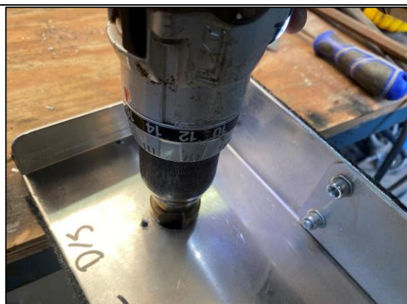
STEP 5 ENLARGE CENTRE HOLE TO 30-32MM (1-1/4") USING THE MOST APPROPRIATE DRILL BIT FOR THE APPLICATION (SPADE BIT FOR WOOD, STEP DRILL FOR SHEET METAL OR APPROPRIATE HOLE SAW).
