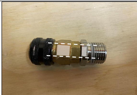
STEP 11 ENSURE THE BULKHEAD AND NITTO FITTING LARGE NUT ARE PARRALLEL. THIS STEP IS VERY IMPORTANT.
