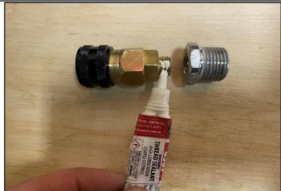
STEP 10 APPLY 567 LOCTITE TO TJM NITTO FITTING (NOT SUPPLIED IN THIS KIT) AND INSTALL TO JBA-CB103 BULK HEAD. THIS WILL BECOME TIGHT TOWARDS THE END AS THE TWO THREADS ARE TAPERED, ENSURE 2 PARTS ARE FULLY TIGHTENED ALL THE WAY.
