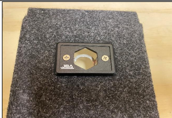
STEP 9 PLACE JBA-CB101A OVER THE HOUSING BRACKET ENSURING THE BRACKET IS SEATED PROPERLY. FASTEN USING M6 COUNTERSUNK SCREWS WITH WASHER AND NYLOC NUT FROM BEHIND.
