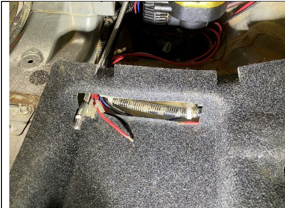
STEP 5.7 FEED THE AIRLINE, SWITCH LOOM AND FUSE WIRES THROUGH THE HOLE JUST CUT IN STEP 5.6
