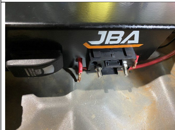
STEP 5.9 FEED THE POWER WIRE THROUGH EITHER SIDE OF THE FUSE, TERMINATE AND HEAT SHRINK.
