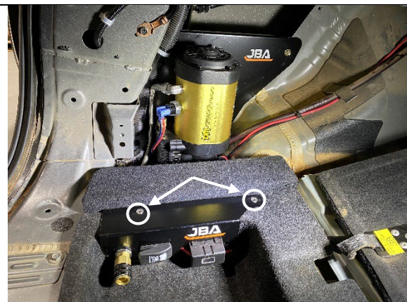
STEP 5.10 INSTALL THE BRACKET TO THE CAPTIVE PLUGS EXPOSED IN STEP 5.5 USING 14G X 1 CSK PHIL SELF TAPPER.
