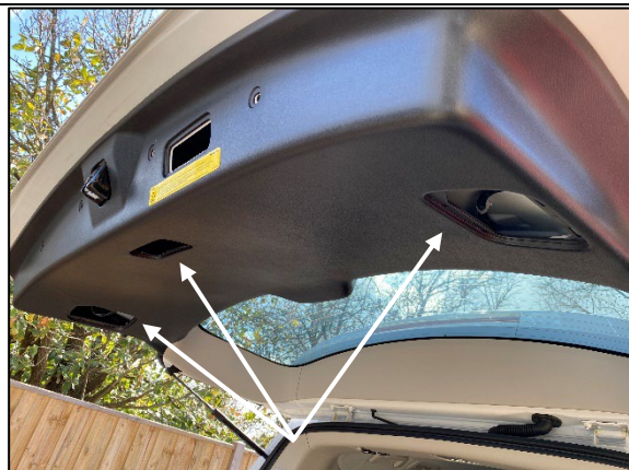
STEP 1.3 REMOVE 3 X PANELS IN TAILGATE GENTLY PRYING DOWN WITH A FLAT BLADE SCREWDRIVER.
