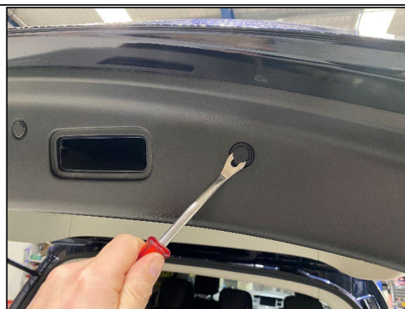
STEP 1.2 USING A TRIM CLIP REMOVER, REMOVE 4 X TRIM CLIPS ALONG TAILGATE.
