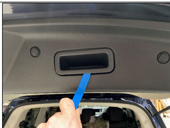
STEP 1.1 REMOVE REAR HANDLE INSERT LEVERING UP FROM BOTTOM USING TRIM TOOL.
