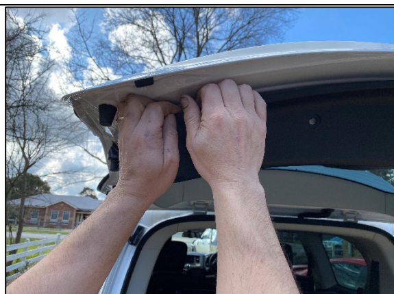
STEP 1.5 START FROM THE CORNER AND BEGIN PULLING DOWN POPPING THE TRIM CLIPS. THESE WILL BE FIRM BUT WILL POP. WORK YOUR WAY ACROSS THE REAR. FULLY REMOVE REAR PANEL AND SIT ON A SOFT WORKSPACE.
