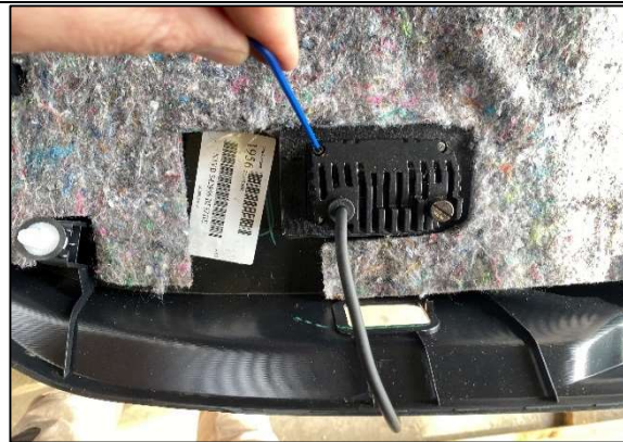
STEP 2.10 FIT THE LIGHT TO THE FASCIA IN THE ORIENTATION SHOWN AND RE-INSTALL 4 X 2.5MM ALLEN KEY SCREWS FROM THE REAR OF THE LIGHT.
