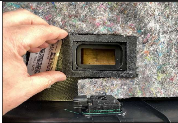
STEP 2.7 FLIP THE PANEL BACK OVER AND FIT THE 10-LB806B REAR RETAINER AND TRIM THE REAR DOOR FOAM AROUND THE LIGHT AS SHOWN.
