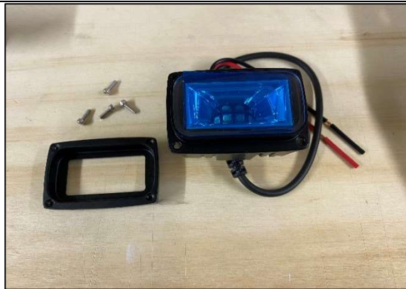
STEP 2.9 SEPARATE THE FRONT FASCIA AND DISCARD (KEEP THE SCREWS).
