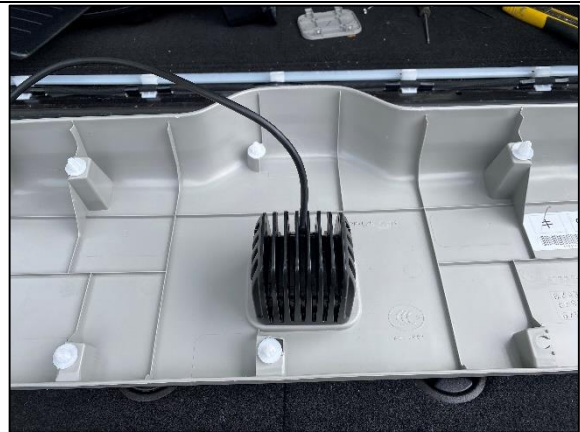
STEP 2.4 PLACE LIGHT OVER FASCIA FROM BEHIND AS SHOWN.
