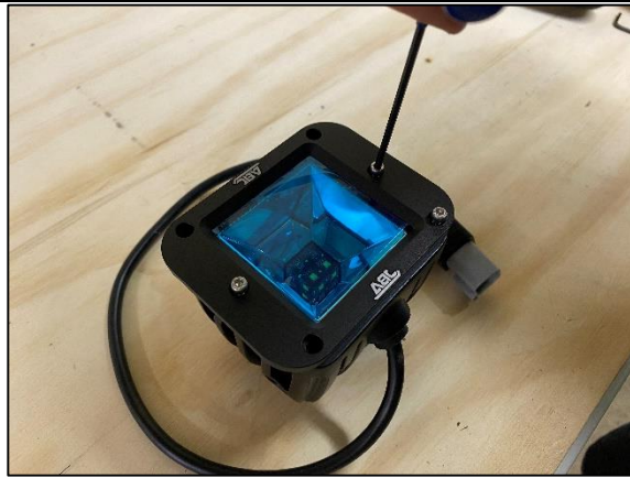
STEP 2.1 REMOVE JBA FASCIA PLATE USING 2.5MM ALLEN KEY.
