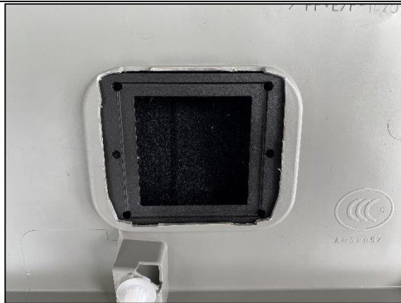
STEP 2.3 PLACE JBA FASCIA IN TO REAR TAILGATE (SHOWN FROM BEHIND IN PIC).
