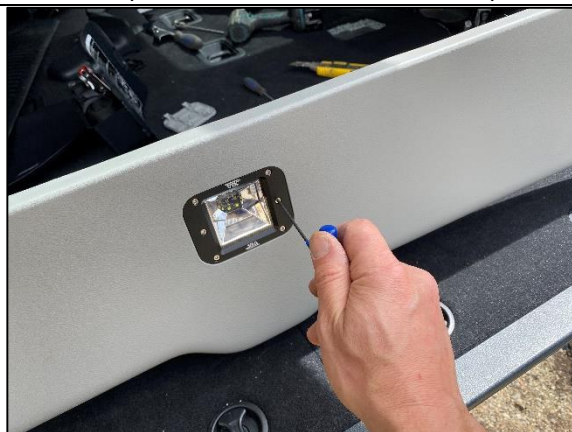
STEP 2.5 RE-ATTACH FASCIA TO LIGHT USING REMOVED SCREWS TO SANDWICH LIGHT OVER TAILGATE AS SHOWN.
