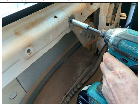
STEP 1.16 IF FITTING A TANK REMOVE THE FORWARD POSITION STEEL PLATE USING 10MM SOCKET X 2. IF NOT FITTING A TANK LEAVE THIS PLATE INSTALLED.
