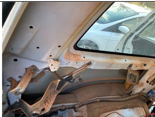
STEP 1.14 FULLY REMOVE THE PANEL FROM THE VEHICLE AND SET ASIDE IN A SAFE PLACE TO ENSURE NO DAMAGE TO THE PANEL.
