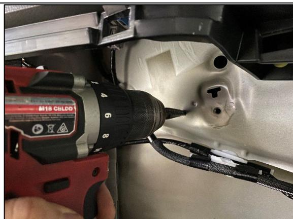
**STEP 1.28** DRILL OUT THE MARKED HOLE TO 7MM AND TREAT EXPOSED EDGES WITH RUST PREVENTATIVE. **BE EXTREMELY CAREFUL TO ENSURE DRILL BIT DOESN'T PULL THROUGH AND DAMAGE OUTER BODY PANEL.**
