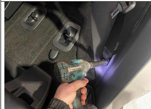
**STEP 1.3** REMOVE THE SECOND ROW SEAT BELT USING 14MM SOCKET.
