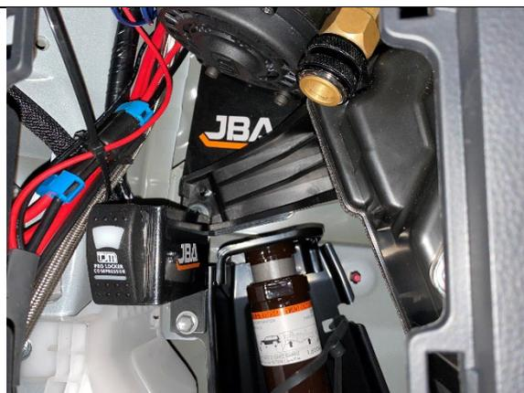
**STEP 3A.2** REMOVE 2 X M6 JACK SCREWS AND INSTALL JBA-231S SWITCH PLATE AS SHOWN USING 10MM SOCKET.
