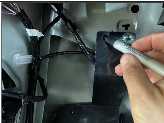
**STEP 1.27** REMOVE FUEL SENSOR ON TOP LEFT AND FIT COMPRESSOR BRACKET IN PLACE LOOSELY FITTING M6 X 20 SEMS SCREWS. MARK THE TOP LEFT HOLE AS SHOWN AND REMOVE BRACKET.
