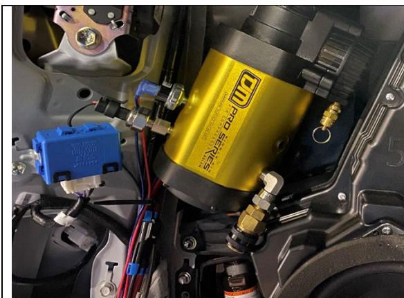
**STEP 3A.1** CHECK CLEARANCE OF NITTO FITTING AROUND SUBWOOFER AND ADJUST AS NEEDED USING 14MM SPANNER.
