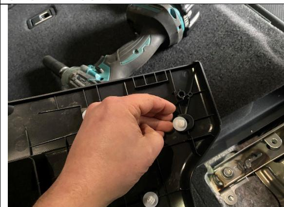
**STEP 1.33** RE-INSERT INTO THE PLASTIC TRIM PANEL LOCATION. THEY WILL NORMALLY SLIDE IN AND POP INTO POSITION. THESE STEPS WILL ENSURE AN EASIER RE-INSTALLATION OF THE PANELS LATER.
