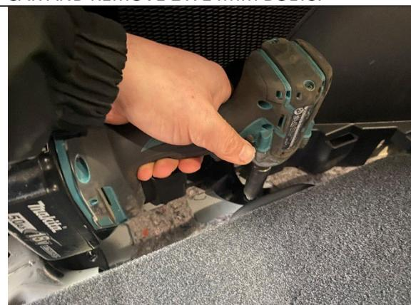
**STEP 1.17** REMOVE 3<sup>RD</sup> ROW SEAT BELT USING 14MM SOCKET AND RETRACT OUT OF THE WAY.
