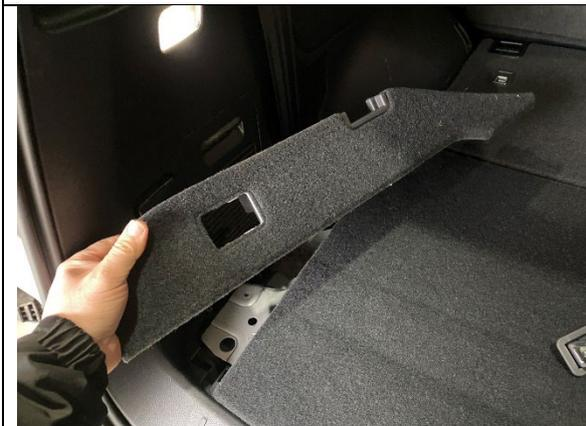
**STEP 1.5** PULL OUT TRIM PANELS (LEFT AND RIGHT SIDES) AS SHOWN. (CHECK FOR ANY TRIM CLIPS THAT MAY HAVE REMAINED IN THE VEHICLE, REMOVE AND REFIT TO THE PANEL SEE STEPS 1.25-1.27).
