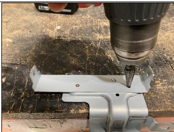
STEP 2.3 USING A 5MM DRILL BIT, DRILL OUT THE SPOT WELDS TO SEPARATE THE TWO SECTIONS OF THE BRACKET.
