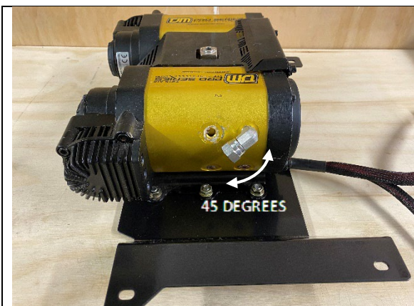
STEP 3.3.1 INSTALL JBA-CB106 90 DEGREE ELBOW TO TOP RIGHT ¼" OUTLET AND FACE DOWN ON A 45 DEGREE ANGLE AS SHOWN.
