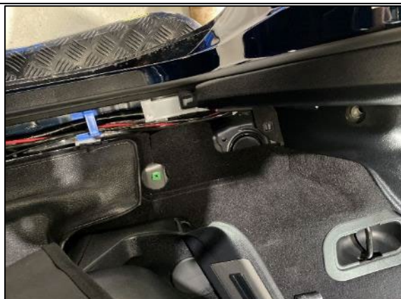
STEP 1.7 REMOVE TRIM PULLING UP FROM FRONT TO REAR.
