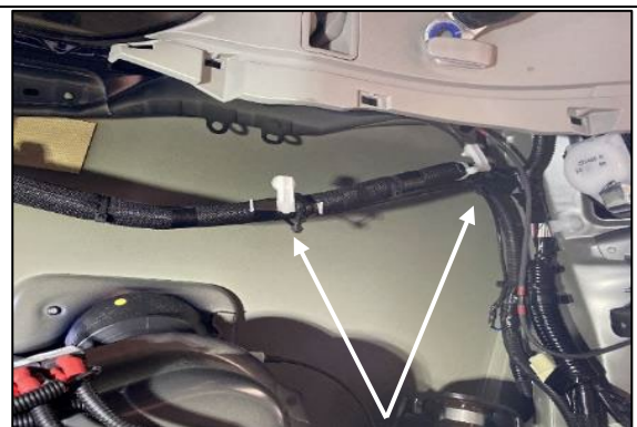
STEP 1.11 REMOVE X 2 PLASTIC LOOM RETAINERS. SQUEEZE FROM BEHIND (FROM SIDES NOT TOP/BOTTOM) AND PULL AT THE SAME TIME TO REMOVE.
