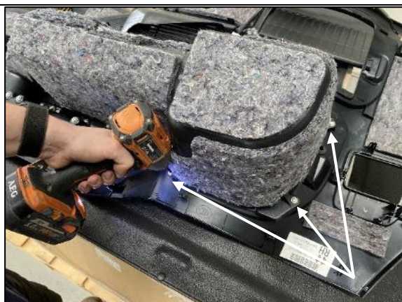
STEP 1.9 REMOVE QUARTER PANEL FROM VEHICLE AND PLACE ON A SOFT, CLEAN SURFACE. FROM THE REAR OF THE QUARTER PANEL, REMOVE THE STORAGE PANEL USING PHILLIPS HEAD DRIVER.
