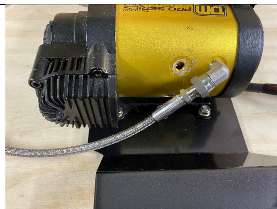
STEP 3.3.2 INSTALL JBA-CB112 800MM HOSE AS SHOWN. (IF FITTING A TANK, HOSE WILL CURVE BACK ON ITSELF- REFER TO STEPS 3.4 BELOW FOR ORIENTATION REFERENCE)
