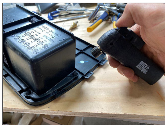
STEP 1.10 IF VEHICLE HAS STORAGE POCKET ON THE REAR OF THE BOTTOM REMOVABLE PANEL, REMOVE THE 5 X PLASTIC WELDS FROM THE REAR. A SMALL BLOW TORCH OR 12MM DRILL BIT CAN BE USED.
