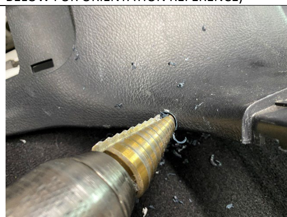
STEP 3.3.4 USING A STEP DRILL, DRILL A 12MM HOLE IN THE PANEL.
