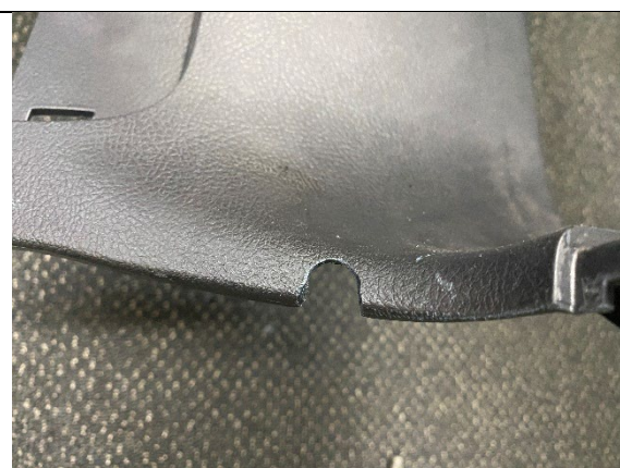
STEP 3.3.6 CLEAN UP AND SHAPE USING RAT TAIL FILE TO CLEAN EDGES AND SHAPE AS REQUIRED.
