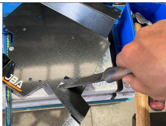
STEP 2.2 FILE ANY TABS LEFT TO ENSURE GOOD FIT FOR SWITCH AND PRESS TJM CARLING SWITCH INTO BRACKET.
