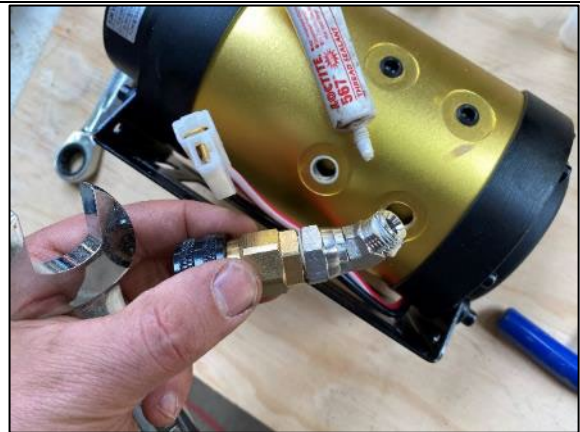
STEP 2.10 FIX THE NITTO FITTING TO THE 45 DEGREE ELBOW SUPPLIED AND APPLY 567 THREAD SEALANT TO THE ELBOW.
