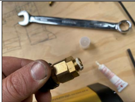
STEP 2.9 APPLY 567 THREAD SEALANT TO THE NITTO FITTING.
