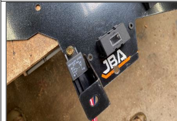
STEP 2.3 ATTACH THE RELAY TO THE M6 NUTSERT ON THE BRACKET USING M6 X 20MM SEMS ASSMSEMBLY.
