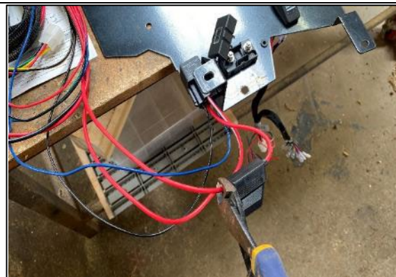
STEP 2.4 CUT OUT THE MAXI BLADE FUSE HOLDER OF THE LOOM. CUT AS CLOSE AS POSSIBLE TO THE FUSE.
