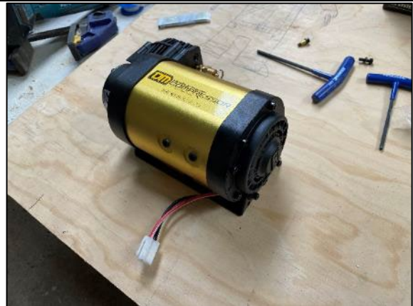
STEP 2.8 ROTATE THE COMPRESSOR 90 DEGREES ENSURING THE POWER WIRES ARE AT THE BOTTOM OF THE COMPRESSOR AS SHOWN
