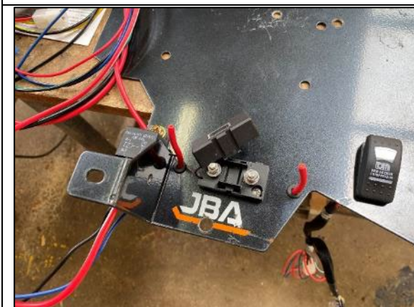
STEP 2.5 FEED THE TRIMMED WIRES THROUGH THE GROMMET FROM THE UNDER SIDE OF THE BRACKET AS SHOWN.
