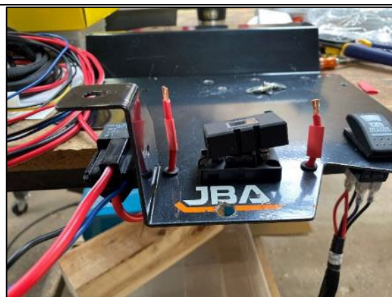
STEP 2.6 STRIP THE ENDS OF EACH WIRE AND SLIDE THE 2 PIECES OF RED HEAT SHRINK OVER THE ENDS
