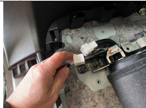
STEP 1.10 UNCLIP THE TWO WIRING LOOMS ON THE PASSENGER SEAT AS SHOWN.
