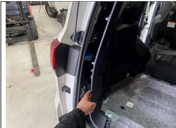
STEP 1.19 START PULLING BACK THE TRIM CLIPS ALONG THE BACK SECTION TOP TO BOTTOM AS SHOWN. (CHECK FOR TRIM CLIPS)
