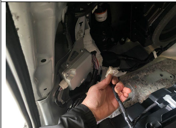
STEP 1.23 MOVE BACK TO THE REAR OF THE VEHICLE AND REMOVE THE MAIN POWER LOOM BELOW THE JACK AS SHOWN.
