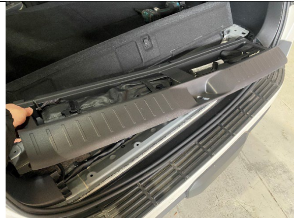
STEP 1.8 REMOVE REAR TRIM PANEL COMPLETELY AS SHOWN. (CHECK FOR TRIM CLIPS)
