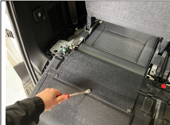
STEP 1.7 FOLD THE PANEL OVER AND REMOVE 3 X TRIM CLIPS AND BOTH LEFT AND RIGHT SEATS TO FULLY REMOVE PANEL.
