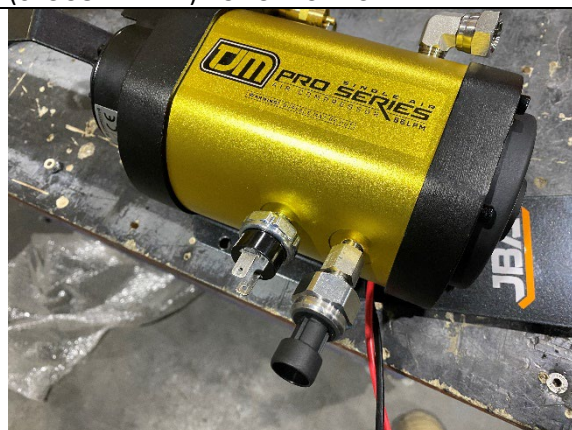
STEP 2A.4 IF FITTING JBA DIGITAL PSI GAUGE, INSTALL PRESSURE TRANSDUCER TO TOP RIGHT 1/8" OUTLET
