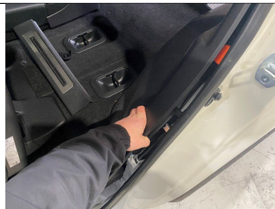
STEP 1.22 MOVE TO THE SECOND ROW PASSENGER DOOR AND PULL THE LAST OF THE CLIPS.
