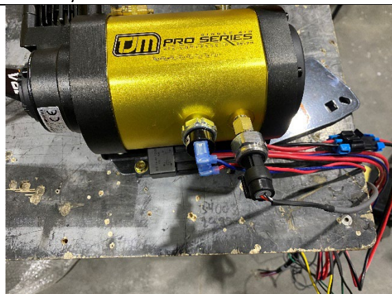
STEP 2A.6 CONNECT THE TJM COMPRESSOR WIRING LOOM TO THE PRESSURE SWITCH AND MAIN POWER AS SHOWN.
