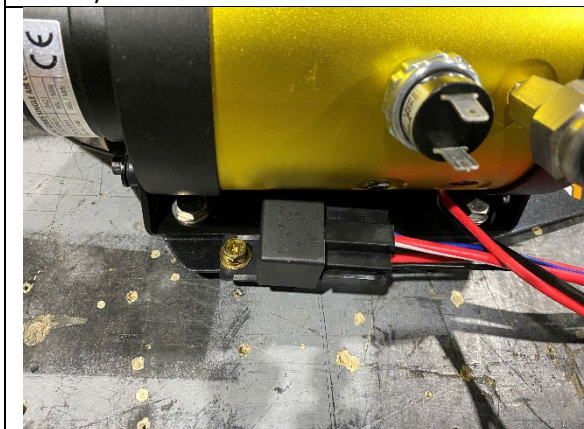
STEP 2A.5 INSTALL THE TJM RELAY TO THE JBA BRACKET USING M4 X 12 PAN AND M4 WHIZZ NUT AS SHOWN
