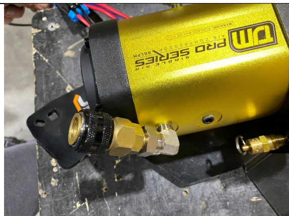
STEP 2A.2 INSTALL THE TJM NITTO FITTING SUPPLIED IN THE TJM AIRLINE KIT (013COMPAKN) PURCHASED SEPERATLEY.
