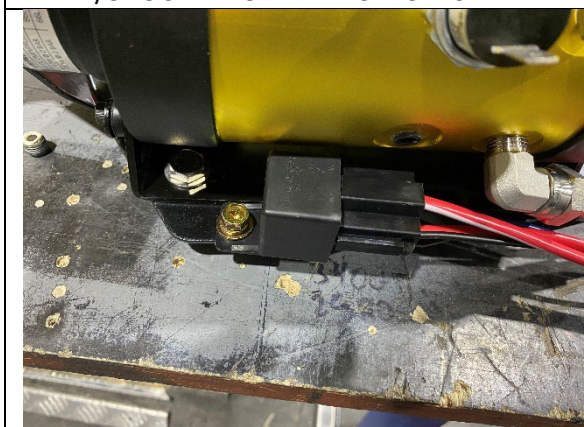
STEP 2B.5 INSTALL THE TJM RELAY TO THE JBA BRACKET USING M4 X 12 PAN AND M4 WHIZZ NUT AS SHOWN
