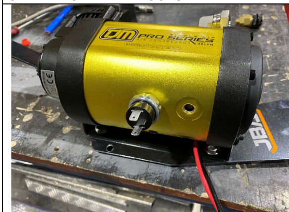
STEP 2A.3 INSTALL THE PRESSURE SWITCH SUPPLIED WITH TJM COMPRESSOR INTO TOP LEFT 1/8" OUTLET ON THE BOTTOM SIDE.
