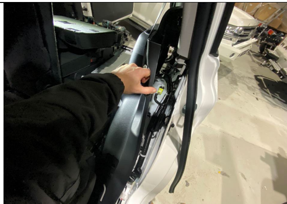
STEP 1.19 MOVE TO THE SECOND ROW PASSENGER DOOR AND BEGIN PULLING BACK QUARTER PANEL AGAIN CHECKING TRIM CLIPS.
