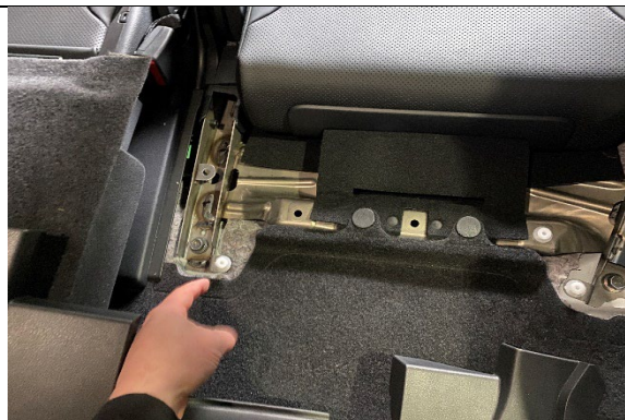
STEP 1.21 REFERENCE PICS FOR TRIM CLIP (EXAMPLE ONLY). AS YOU ARE REMOVING PANELS, KEEP NOTICE OF ANY CLIPS THAT HAVE REMAINED IN THE VEHICLE- NORMALLY WHITE OR GREEN AS SHOWN.
