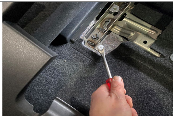
STEP 1.22 USE A TRIM CLIP REMOVER TO POP OUT OF THE VEHICLE AS SHOWN.
