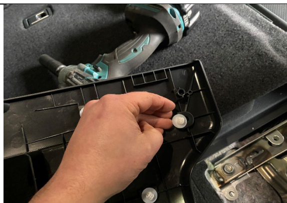
STEP 1.23 RE-INSERT INTO THE PLASTIC TRIM PANEL LOCATION. THEY WILL NORMALLY SLIDE IN AND POP INTO POSITION. THESE STEPS WILL ENSURE AN EASIER RE-INSTALLATION OF THE PANELS LATER.
