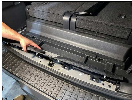
STEP 1.1.10 REMOVE THE REAR PLASTIC TRIM. CHECK FOR ANY TRIM CLIPS LEFT IN THE VEHICLE.
