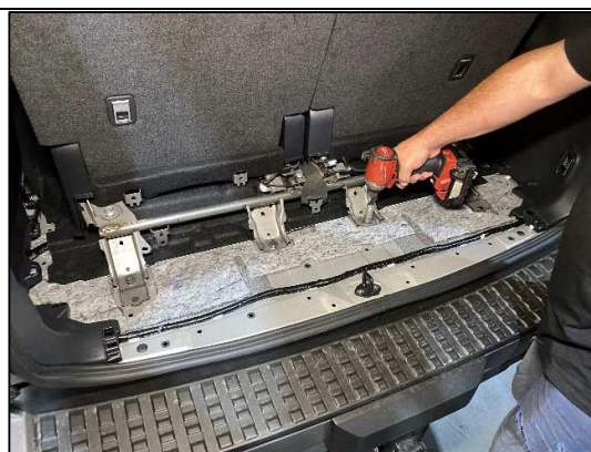
STEP 1.1.12 REMOVE 4 X 14MM BOLTS EXPOSED AS SHOWN AND SET ASIDE.
