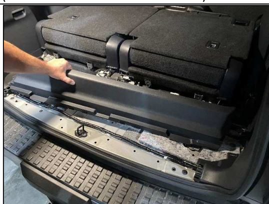
STEP 1.1.11 REMOVE THE PLASTIC TRIM COVER AS SHOWN. CHECK FOR TRIM CLIPS.
