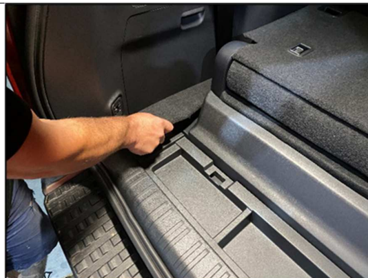
STEP 1.1.8 REMOVE THE LEFT AND RIGHT TRIM PANELS.
