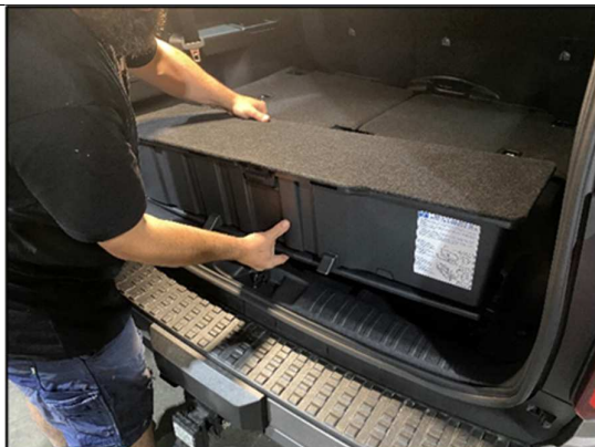
STEP 1.1.7 MOVE TO THE REAR OF THE VEHICLE AND REMOVE THE REAR STORAGE BOX.
