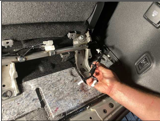
STEP 1.1.13 REMOVE THE 2 BODY CLIPS FOR THE SEAT WIRING LOOM AND UNCLIP AS SHOWN.
