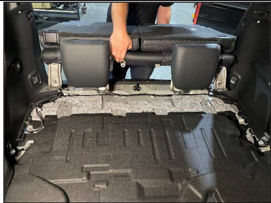
STEP 1.1.14 FOLD THE SEAT DOWN AND LEFT OUT OF VEHICLE (2 PEOPLE IS BEST TO ENSURE TRIM ISN'T SCRATCHED WHEN LIFTING OUT)
