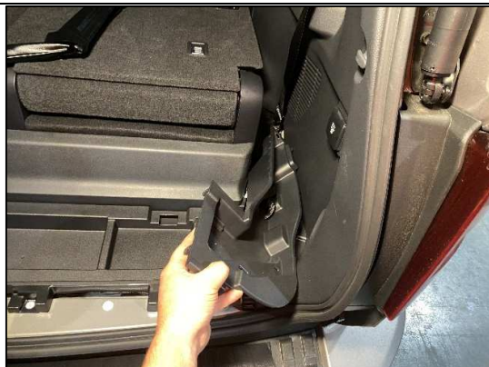
STEP 1.1.9 REMOVE THE LEFT AND RIGHT PLASTIC STORAGE SECTIONS. THE DRIVERS SIDE LIFTS UP WITH TRIM CLIPS, THE PASS HAS TABS (FOLLOW INSTRUCTIONS ON PANEL)
